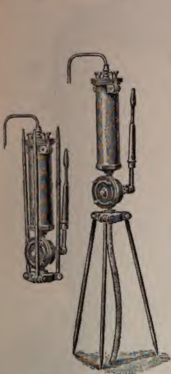
FIG. 51.—Berkefeld filter with pump for field use. (Munson.)
